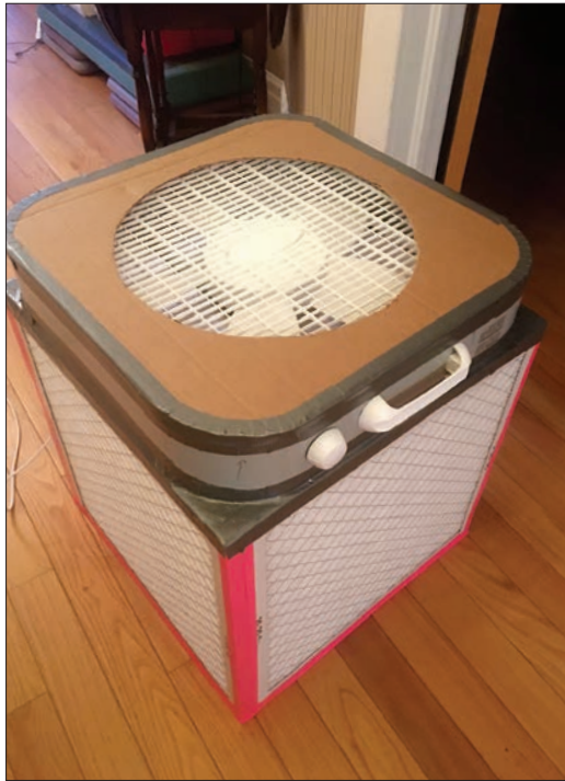
The do-it-yourself Corsi-Rosenthal Box can provide commercial-quality air purification for a fraction of the cost.
