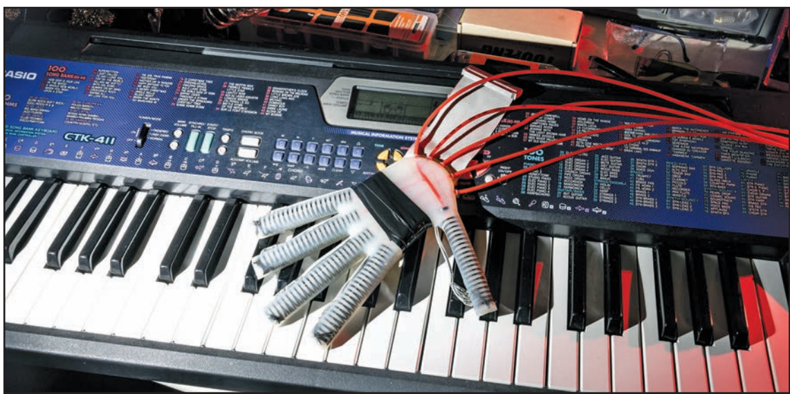
The soft robotic glove integrates five actuators into a single wearable device that conforms to the user's hand.
